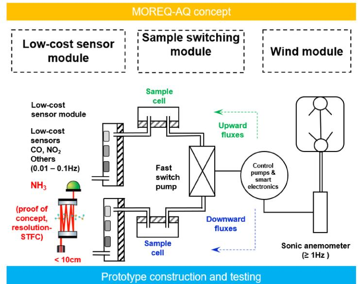
Figure 1: Schematics of prototype modular relaxed eddy instrumentation. The three modular units that comprise the design are shown in the figure
