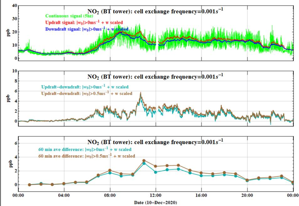
Figure 3: Example data for NO<sub>2</sub> BT Tower London, (a) continuous real data from high grade reference instrument at 5Hz (green), simulated signal expected in updraft and downdraft component (blue and red respectively), (b) difference between the updraft and downdraft signals (a measure of flux) with- (brown) and without a dead band (cyan), (c) hourly averages of the signal shown in (b).
