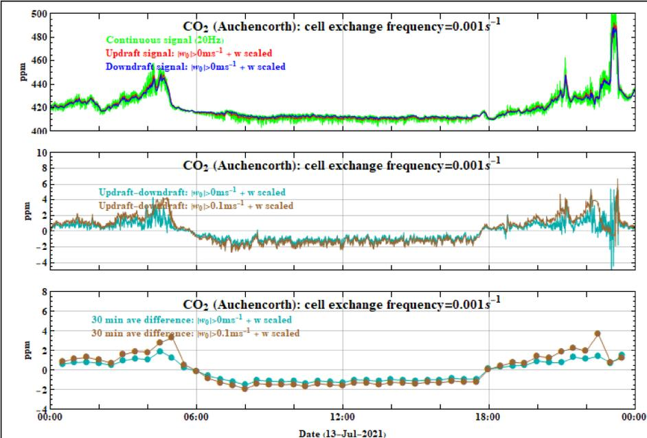
Figure 2: Example data for CO<sub>2</sub> at Auchencorth Moss field CEH, (a) continuous real data from high grade reference instrument at 20Hz (green), simulated signal expected in updraft and downdraft component (blue and red respectively), (b) difference between the updraft and downdraft signals (a measure of flux) with- (brown) and without a dead band (cyan), (c) hourly averages of the signal shown in (b).
