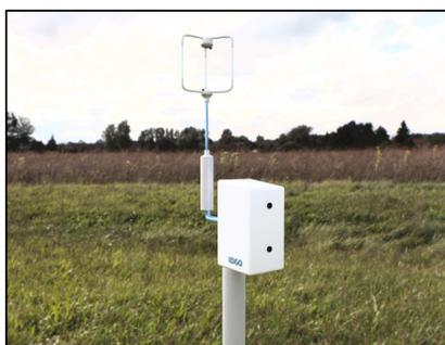
Figure 6: Rendering of a MOREC-AQ unit shown to size relative to a typical 3-D sonic anemometer
