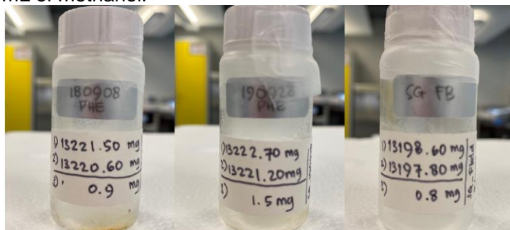
Figure 1. Biomass burning aerosol samples. From left to right: non-wildfire, wildfire, and field blank.
